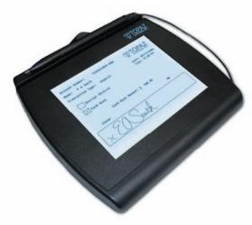
Interactive LCD pads for displaying text, graphics, and pen-tap checkboxes
