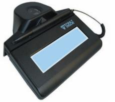
Integrated electronic signature and fingerprint capture
